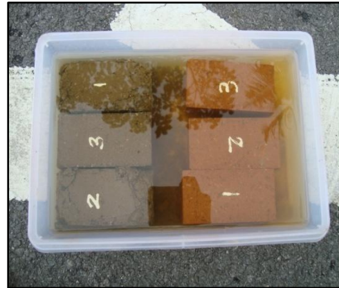
Rajah 10: Ujian kadar serapan air
